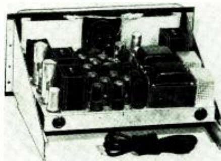
The picture above shows the Ward amplifier with both 45-watt power chassis installed. Operated in parallel, they furnish 90 watts.
