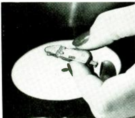
The ceramic crystal pickup made by Sonotone.
