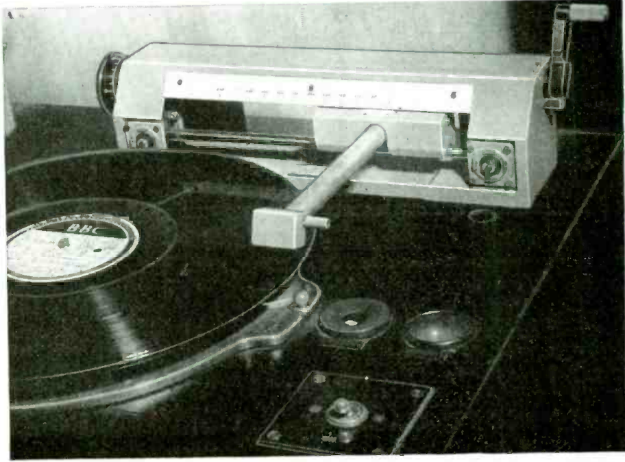
Fig. 2—With this device the operator can "tap in" or find any desired point on a recording.
