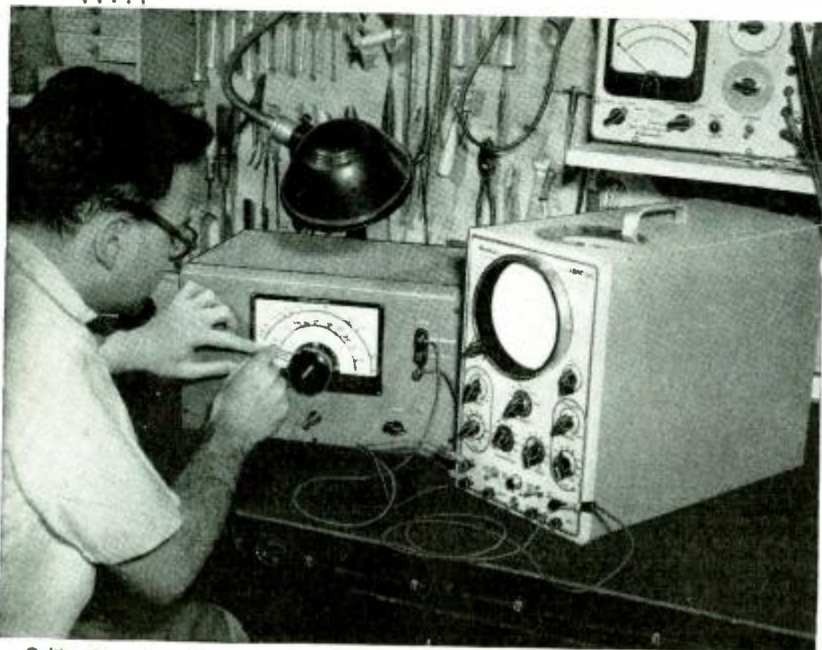
Calibration set-up. Our author is making a careful pin-prick mark through the dial pointer.
